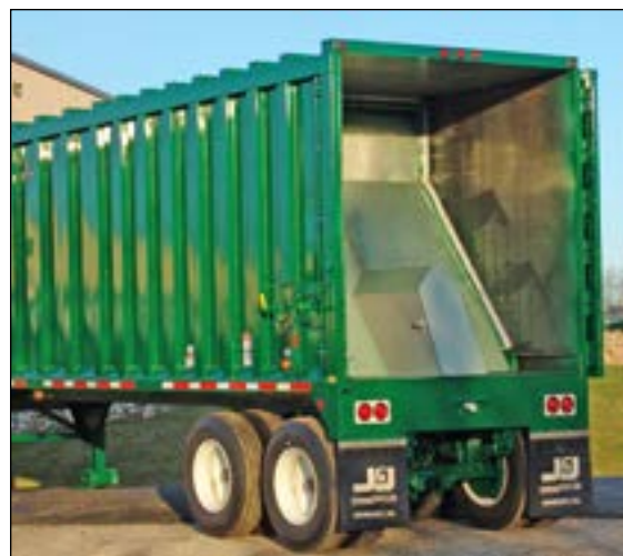
Ejector ram cylinder is sized to completely unload trailer and the replaceable UHMW wipers on top and sides of ejector ram provide superior clean-out.
