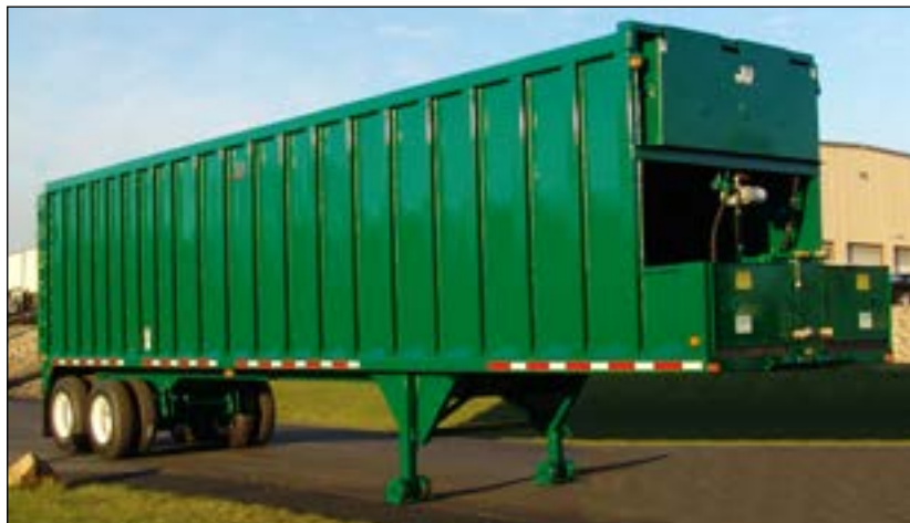
Tractor hook-ups and hydraulic controls located in one area for ease of operation. Trailer shown with optional trailer mounted hydraulic tank.
