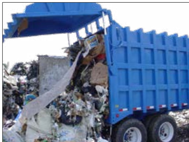
Fully self-contained trailer shown with auxiliary engine, retractable roof and hydraulic lift and lock compactor tailgate.
