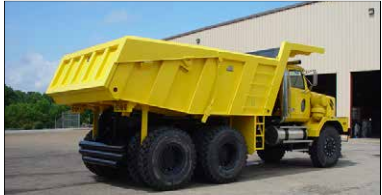
The low profile sides are designed for easy and efficient loading with a scowled end to secure large boulders and reduce hydraulic cylinder stress upon boulder impact.
