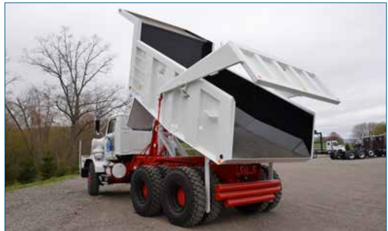
The auto lift tailgate maximizes material loading while the full cab guard protects the operators in the cab from falling debris.
