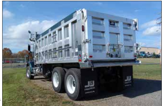
In addition to the optional combination tailgate shown here, air operated high lift gates are also available.
