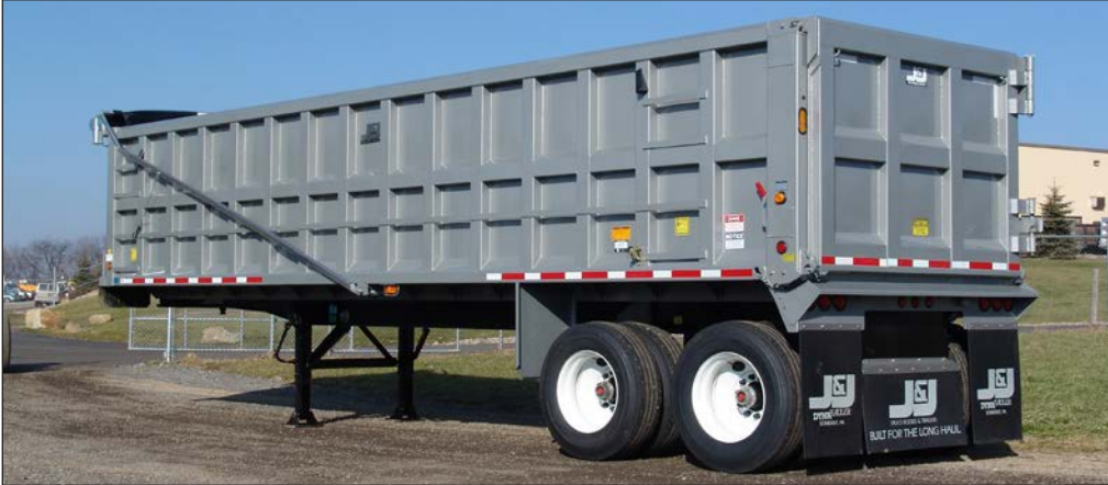
Convert from conventional gate to a side swing gate in two quick steps with our easy-to-use, optional combination tailgate.
