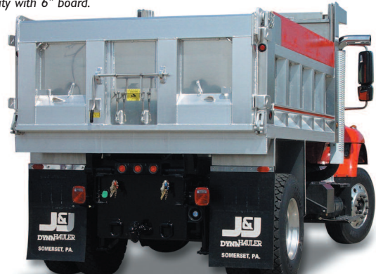
Medium duty dump bodies feature 9 - 12 foot aluminum or steel beds.
