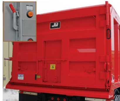
Optional 3-way barn door style tailgate features a ground control release for fast and easy opening.
