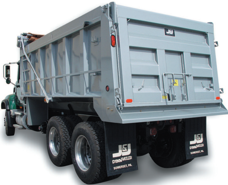
Crossmemberless body greatly reduces the weight of these trucks.
