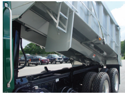
Crossmemberless body greatly reduces the weight of these trucks.
