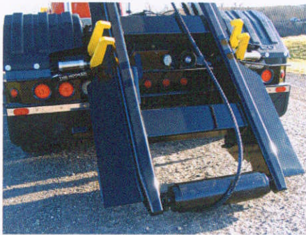
Heavy-duty, replaceable tail rollers, inside and outside controls for easy access and heavy-duty stops are standard features on J&J roll-off trucks.
