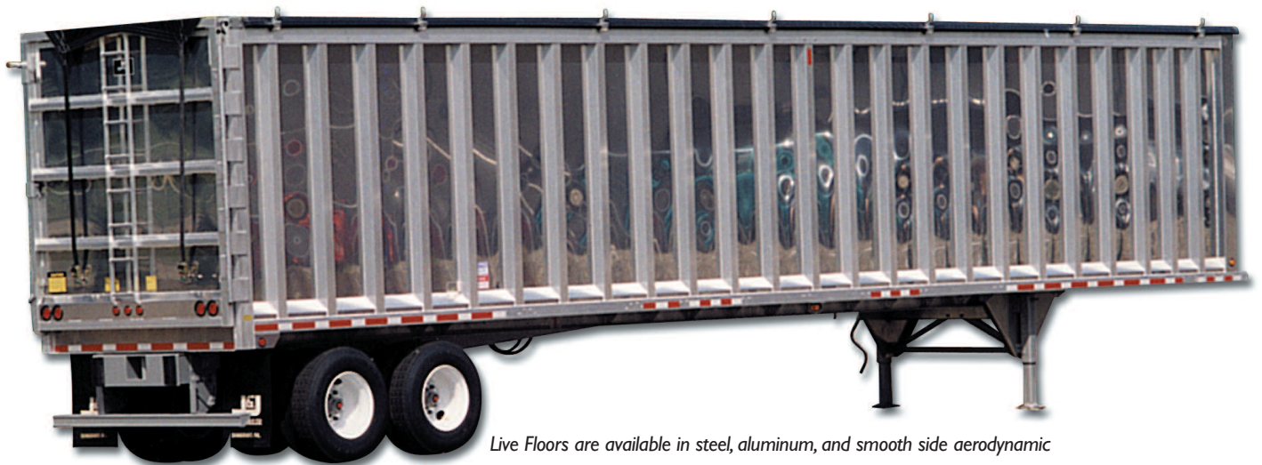
3/4 inch thick top rail and roller style cross tie combine for the strongest top loading trailer available (aluminum)
