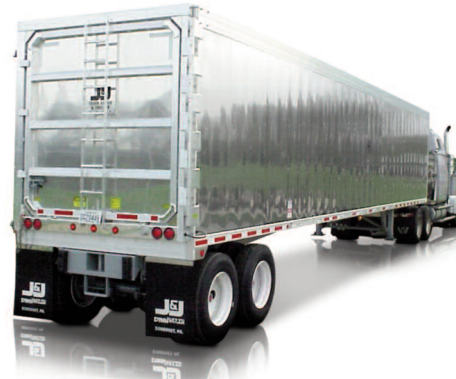
Aerodynamic Smooth Side Series (one sheet with no seams)
